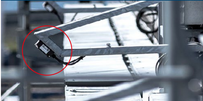
Fig 4: Anchors / receivers mounted on a gantry crane
