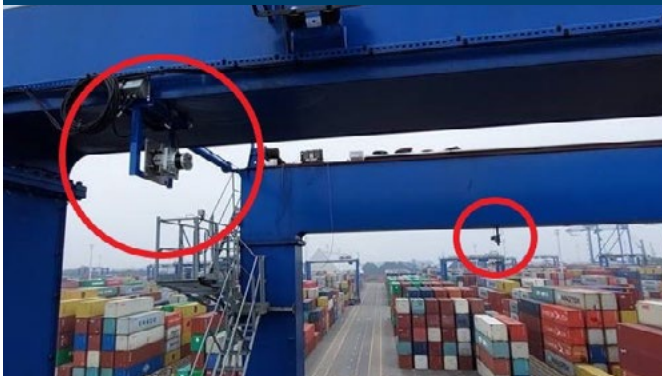
Fig 11: Scanner mounting positions on an RTG
