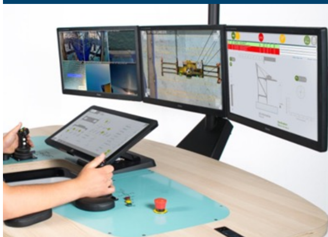
Fig 22: Example for remote operator desk showing live video streams
