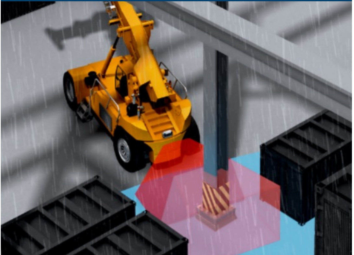
Fig 7: Spatial perception of 3D stereo camera in the port environment
