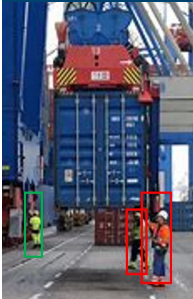
Fig 25: Example for people detection on a remote operator desk including zones to provide additional warnings
