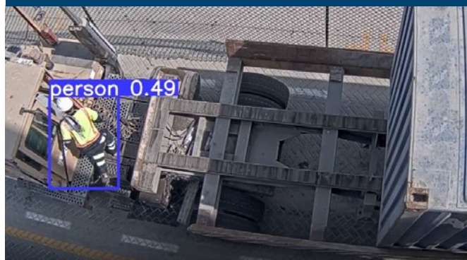
Fig 26: Example of people detection with the probability of detection
