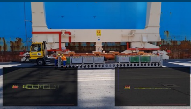
Fig 16: Truck positioning actual picture and 3D-Point Cloud
