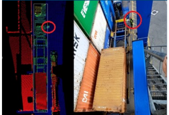
Fig 5: 3D-Point Cloud and an actual picture of the area (subject beside the truck in red circle)
