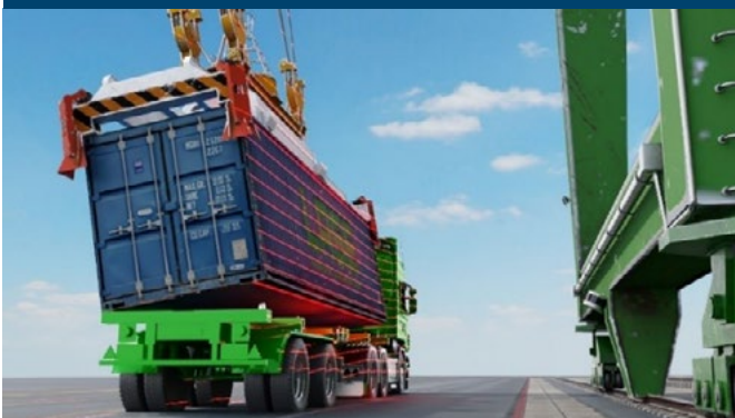
Fig 8: 3D-Scanlines on the side of the vehicle
