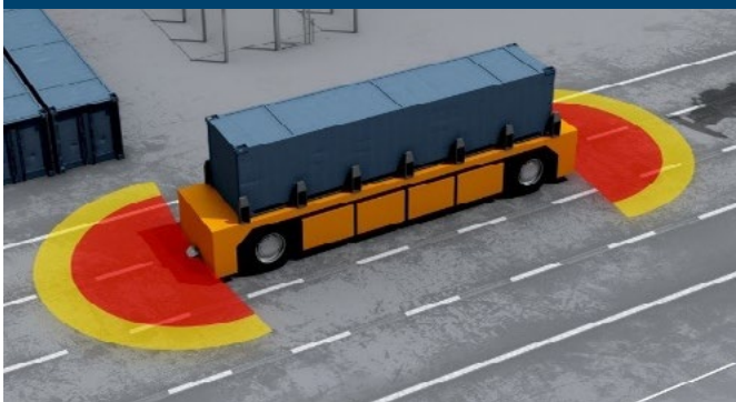
Fig 26: AGV collision prevention with 2 x 2D-Laser scanning to both sides
