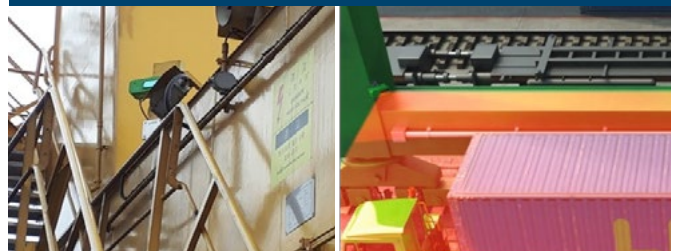
Fig 7: Mounting Positions of the 2D-Laser Red horizontal light curtain (right picture)
