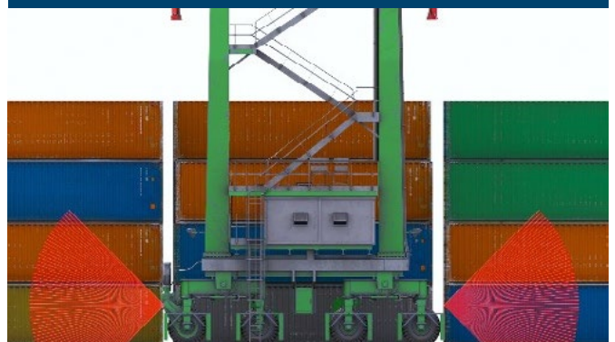
Fig 29: 3D-Laser view into gantry drive direction for Gantry Collision Prevention
