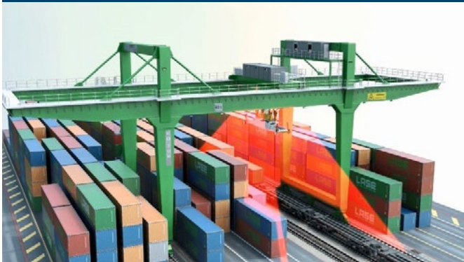
Fig 23: Image with scan-plane of 2 x 3D-Laser to measure the wagon position
