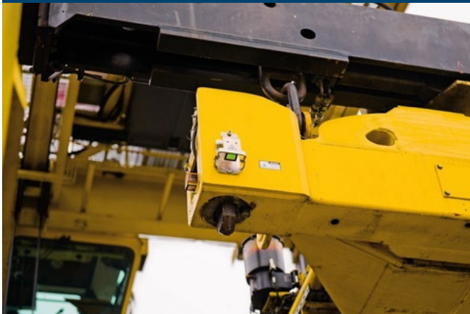
Fig 4: 1D-Laser on the spreader
