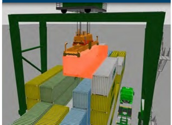
Fig 21: Possible occurrence of a collision, therefore surveillance cube around the load is red and the crane has stopped moving
