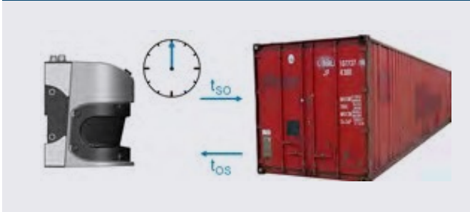
Fig 32: 2D-Laser measurement principle time-of-flight
