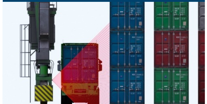
Fig 28: 3D-Laser view into the truck lane for Truck Lifting Prevention
