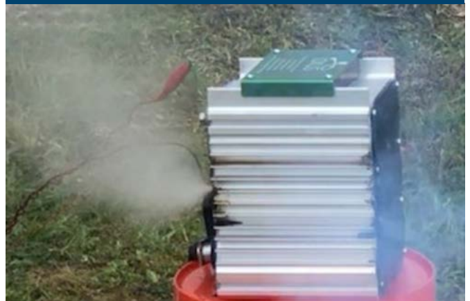
Fig. 8: Ultracapacitor Under Overvoltage Test
