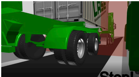
Image 12: Scan plane in red. Motion has been stopped by the indicator that trailer is going upwards together with the container.
