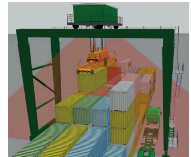
Image 10: With 2 x 2D-laser scanner bays can be scanned. Additionally, laser scanners measure reference marks on the headblock. By comparing the position of both objects containers in yard and the load position a collision in the bay can be prevented.
