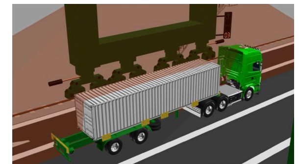
Image 5: A scan plane "cuts" the container determining the front, rear and centre of the container. The truck driver receives feedback about his position in relation to the centre of the crane via a digital display.
