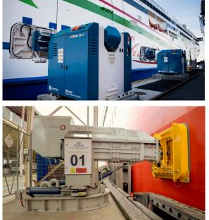
The technology has been in use since the 90s and has been installed at bulk, container handling, Ro/ Ro, passenger and lock applications worldwide. At date of this publication, vacuum mooring installations have completed more than 750,000 mooring operations entirely without incident, including the regular mooring of 19,000-TEU vessels.
