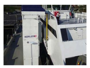
Since many automated mooring systems enable fast and stable positioning relative to the shore, they are commonly used together with (automated) power supply systems. The fast connection to clean power reduces emissions and increases the charging time for electrical vessels. The higher vessel stability simplifies the technical requirements of the connection solution, making it safer and more efficient.
