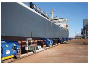
Though a bulk carrier port, Port Hedland faced multiple challenges during operations. Both passing ship effects and high tides changes impacted the feasibility and efficiency of loading operations at the port. This required the automated mooring units to be installed on the wharf face and on rails to fully follow the ship during draft and tide changes. This is especially critical for this application due to the extended time the vessels spend at berth during loading.
