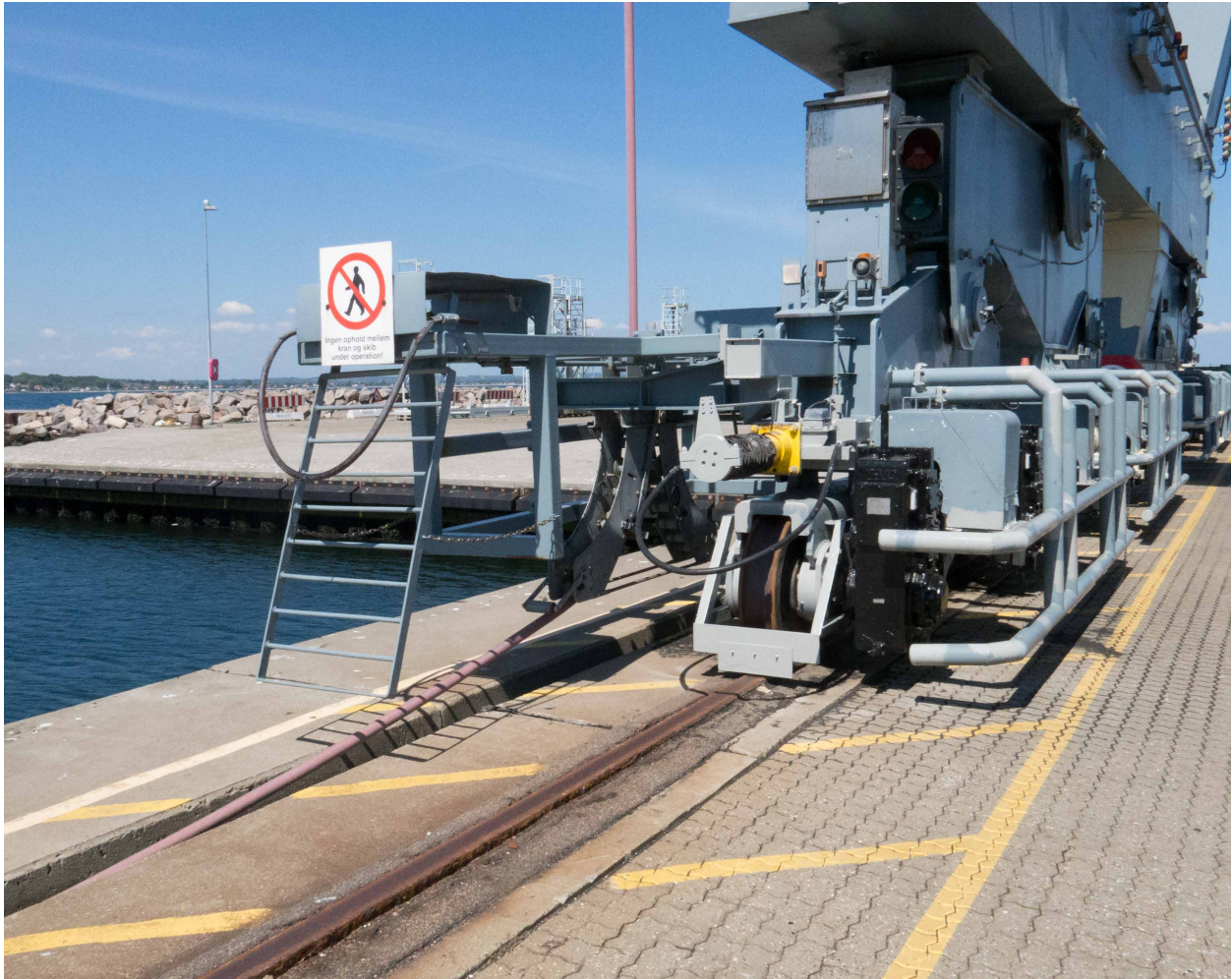
Photograph J: STS crane gantry, wheel, rail, cable, trench, and crane buffer
