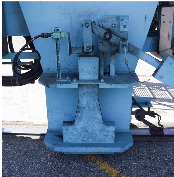
Photograph F: STS crane stowage pin
