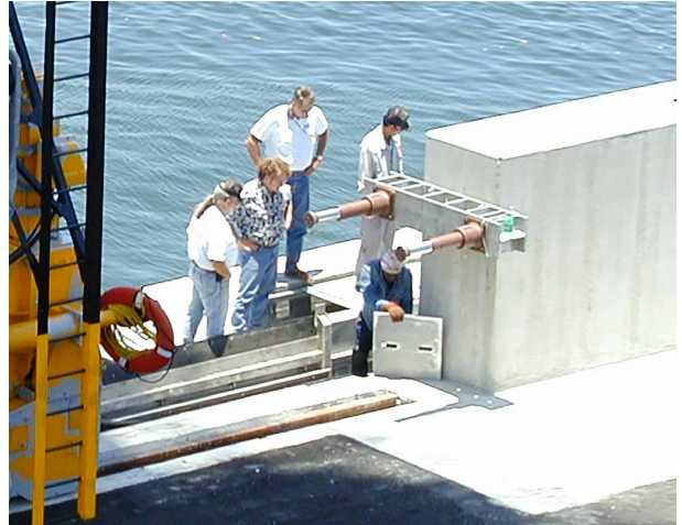
Photograph M: STS crane end stop with twin hydraulic buffers
