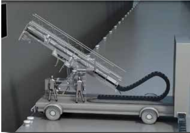
Picture 15: A CMS for cruise applications using a telescopic bridge system to reach the connection point, and a chain system to adjust to tidal and weather conditions
