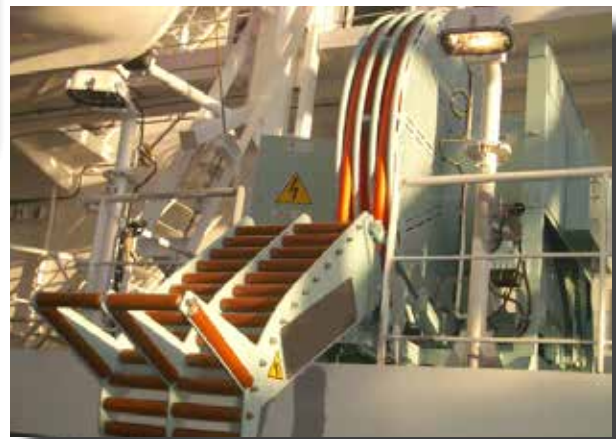
Picture 10: Cable reel using a slip ring
