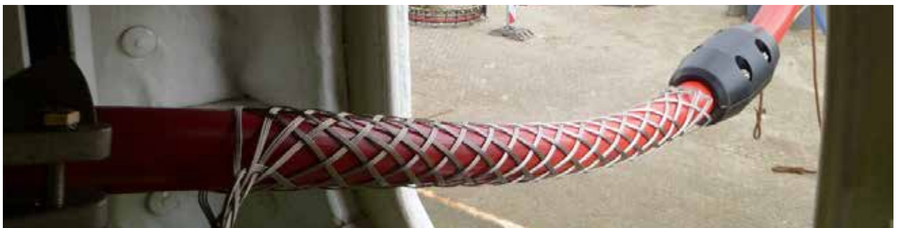
Picture 3: Example 11 kV plug for Ro/Ro and LNG ships up to 6.5MVA with a single cable
