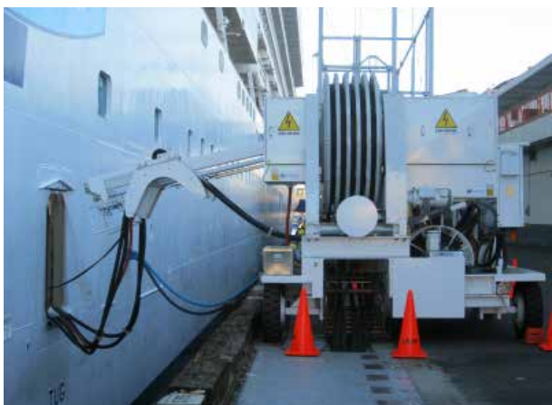
Picture 19: CMS integrated into a semi-movable container
