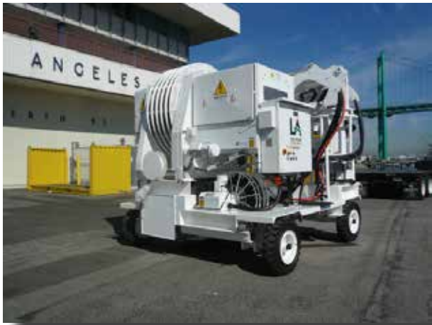
Picture 7: A cable reel system and crane device mounted on a trailer
