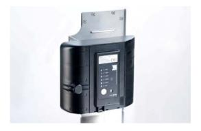
An RFID-based Container Security Device *Source: IDENTEC SOLUTIONS*
