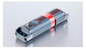
Above, an RTLS active RFID tag. Below, an active beacon-type tag. *Source: IDENTEC SOLUTIONS*
