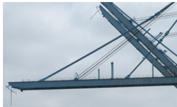
Picture 3.49: Forestays of three monogirder cranes. Sagging and straightening of the stays, due to loading and unloading the boom, results in stays bouncing up and down, which increases fatigue cycles of load.
