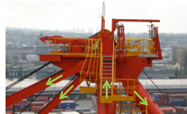
Picture 3.60: The same beam from the side with arrows showing typical forces at the apex.
