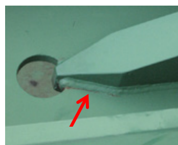
Picture 3.50: A crack in the weld at the end of a forestay connection plate—in spite of stress relief hole. The relief hole reduces the stress concentration but does not eliminate it.
