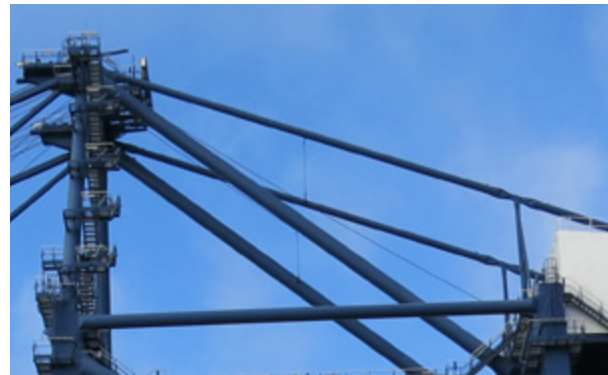
Picture 3.40: Typical arrangement for twin girder crane, backstays above the upper diagonals.
