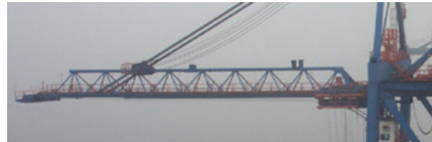
Picture 3.28: Truss boom.
