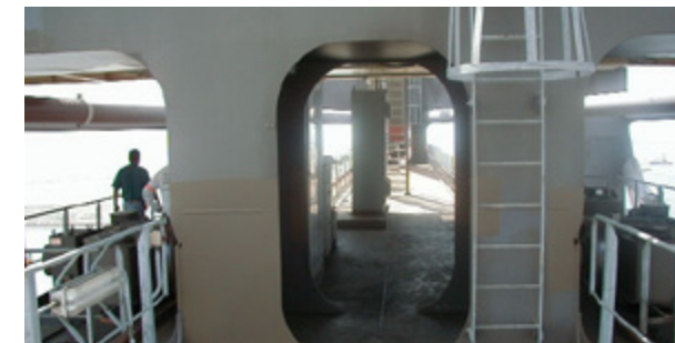
Picture 3.21: Welded LS TGSB connection to monogirder boom. Notice the large radii at the transition.
