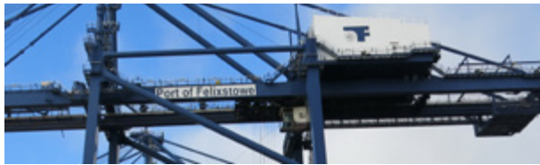
Picture 3.26: Trolley twin girder.
