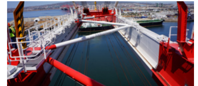
Picture 3.35: Twin girder boom with typical diagonal bracing for lateral stiffness.
