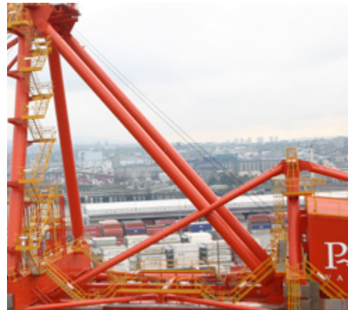
Picture 3.39: Upper diagonal connecting to forestay at the top trolley girder at bottom.
