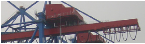
Picture 3.25: Trolley monogirder.
