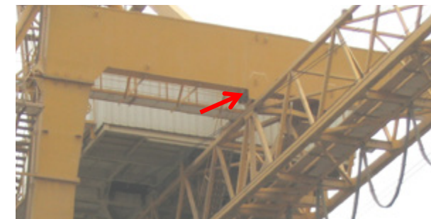
Picture 3.22: LS TGSB of a truss boom crane, in this case without radii at the points of transition.
