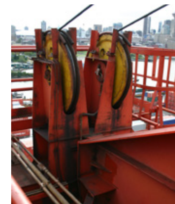
Picture 3.71: Main hoist sheaves at the backreach. These structures are fracture critical.
